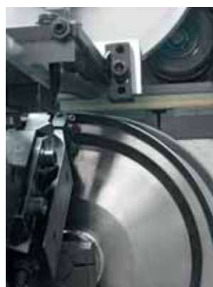
TWINFEELER No compromise on the finish with track feeler + pre-track feeler staggered for high speeds. xd
