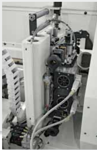
R-E Movements on linear guides with recirculating balls. xd
