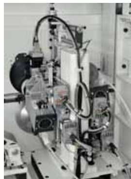
RSU-E Minimum interaction with the panel due to movements on linear guides with recirculating balls. xd
